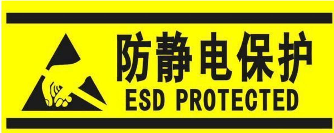
Electronic components and circuits are very sensitive to electrostatic discharge, although the company will design the main interface on the board card to do anti-static protection design, but it is difficult to do anti-static safety protection for all components and circuits. Therefore, it is recommended that you take ESD safety measures when handling any circuit board component.
